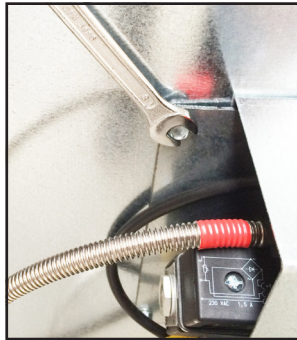
unscrew 4 screws in the corners (key 8)
